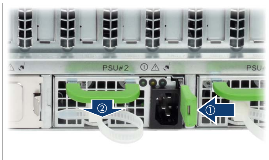
Figure 14: Unlocking and removing the power supply unit
